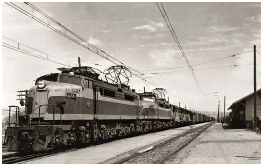
FIGURE 9.8: On the Milwaukee Road, passenger and freight trains alike were powered over mountain passes by electric current generated by giant motors. On the down grade, the motors were reversed and acted as dynamos (machines that convert mechanical energy into electric energy) and returned power to the lines.
